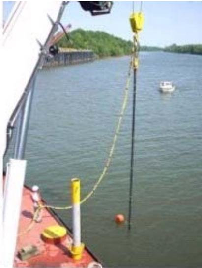
Vibratory Core Sampler
