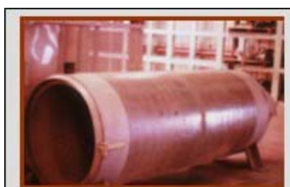
Killen, Ohio Power Plant Intake Pipe Made of Wedge Wire
