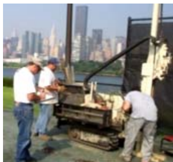
Soil and Groundwater HazMat Sampling with a Geoprobe
