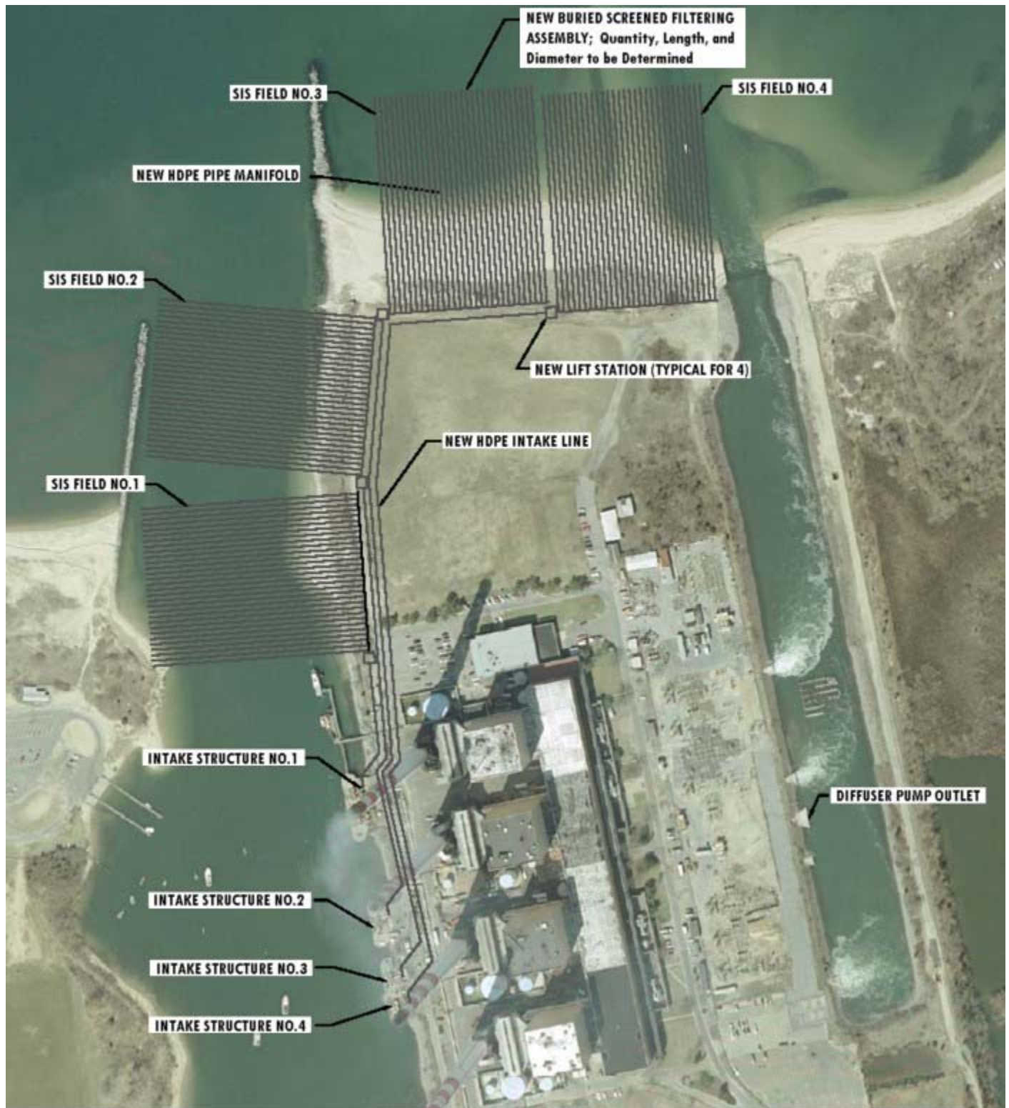
Aerial View of a Typical SIS Design
