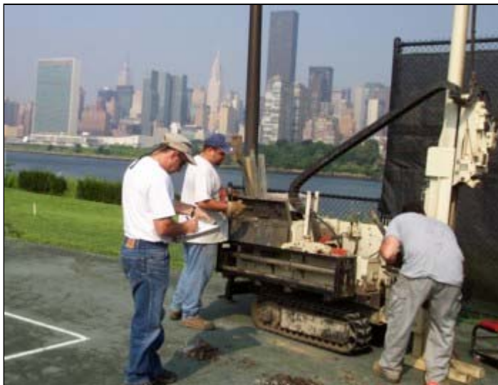
Soil and Groundwater Sampling with a Geoprobe
