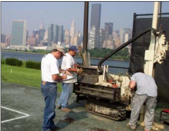
*Soil and Groundwater Sampling with a Geoprobe*
