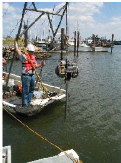
Lowering the vibracorer in the James River near Richmond
